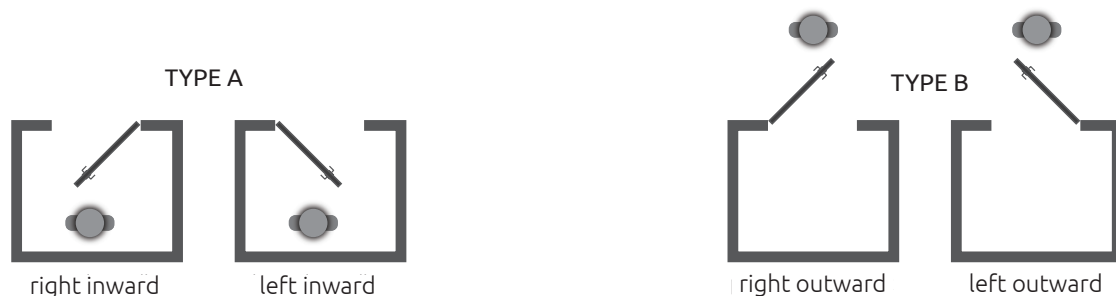
Fig. 4 – PIU DOORS OPENING DIRECTIONS ACCORDING TO FRAME TYPE A I TYPE B
